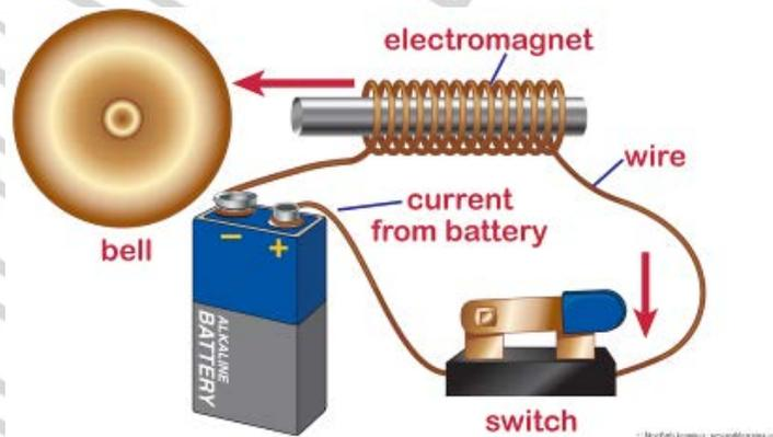
The magnetic field produced here when the circuit is closed is a combination of the magnetic force from the electrical current and the metal bar. Opening the circuit reduces the strength of the magnetic field and stops the clapper from striking the bell.
