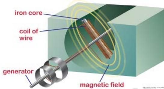
Generators produce almost all of our electricity. By burning coal, oil or natural gas, large amounts of water are converted to steam which provides the mechanical energy needed to turn the generators. In some cases, falling water alone is enough to do this job.
