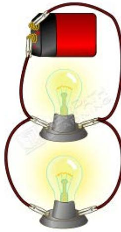
In a **parallel circuit**, if one bulb goes out, the other bulb will stay lit.
