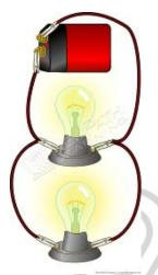
In a parallel circuit, if one bulb goes out, the other bulb will stay lit.
